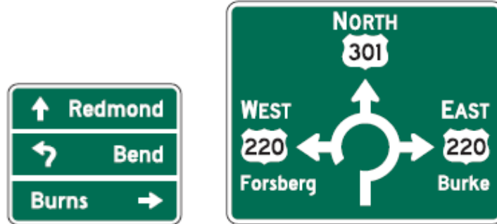
Figure 2.2 Conventional and diagrammatic advance guide signs at roundabouts (from the proposed 2009 MUTCD).
